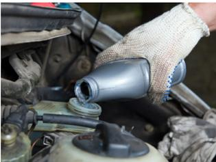
The Solution: Completely flush the system of old brake fluid.
